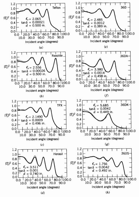
**Figure 4.2** The measured power transmission for different dielectric samples is shown by the dotted lines. The line curves are the calculated  $|T_{\perp}|^2$  using the best-fit estimates of  $\varepsilon_r$  and tan  $\delta$ . [From Shimabukuro et al. (1984).]
